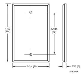
Fig. 1. C7772 Dimensions in in. (mm).
